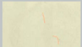
orange protective fibres spread randomly across entire paper surface
