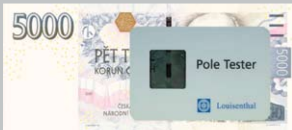
Pole Feature — hatching with lighter and darker rhomboids — appears on security windowed thread when Pole Tester is applied
