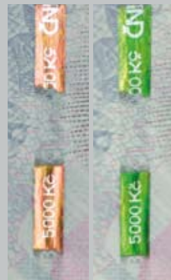
silvery security windowed thread changes colour from purple to green when tilted
