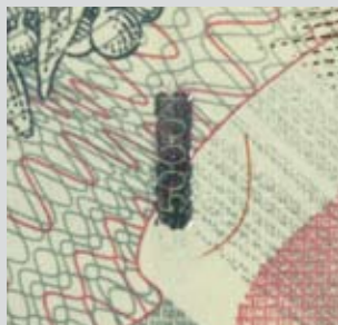
no effect on security windowed thread when Pole Tester is applied
